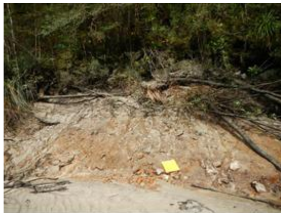
Figure 3-16: Sediment clasts expelled from bank due to high water pressure in saturated bank.
