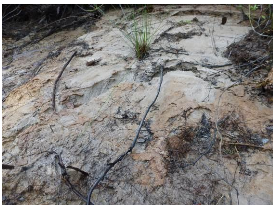
Figure 3-21: Tension cracks and bank slumping in zone 5.
