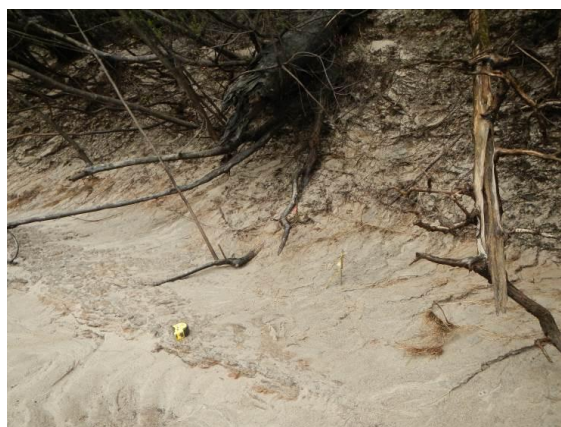
Figure 3-13: Break in slope on bank at erosion pin site 3A showing scour of root mat and lack of deposition of organic matter in spring 2013.
