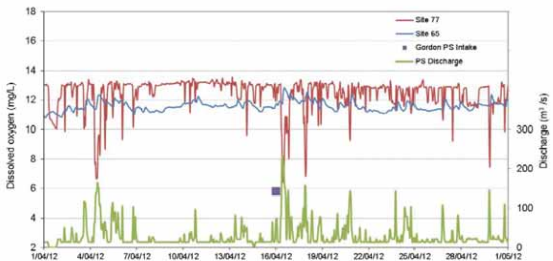
Figure 3-8 Dissolved oxygen concentrations at site 77 (tailrace) and site 65 (compliance site) relative to power station discharge 1–30 April 2012
