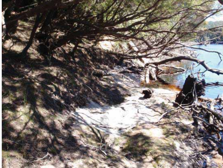
Photo 4-5 Sediment flows in 1–2 turbine bank level at erosion pin site 2H. White sands are being transported from under deteriorating root mat
