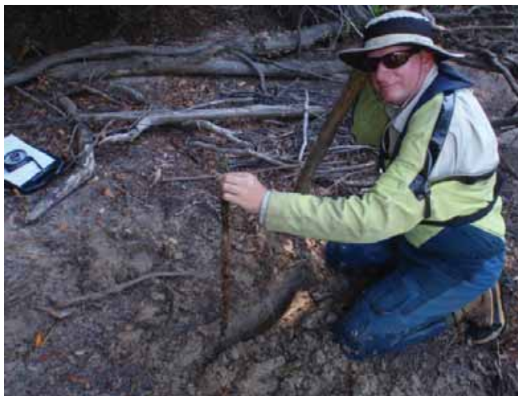
Photo 4-15 Recovery of scour chain at site 5F with help of metal detector
