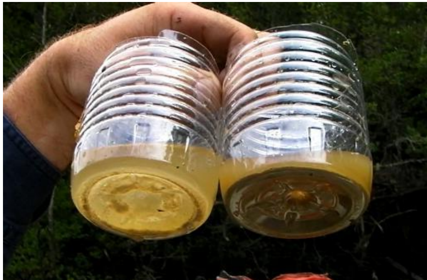
Photo A5-6 Photo showing increase in sediment content of water as it flows down sandy bank toes. Water on left collected near top of bank, water on right collected where water entering river. Vertical distance between ground water level and river level estimated to be 1 m. Distance over bank ~ 2.5 m
