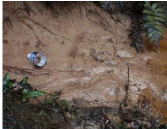
Photo A5-4 Initial, diffuse draining of bank during drawdowns and ramp-downs
