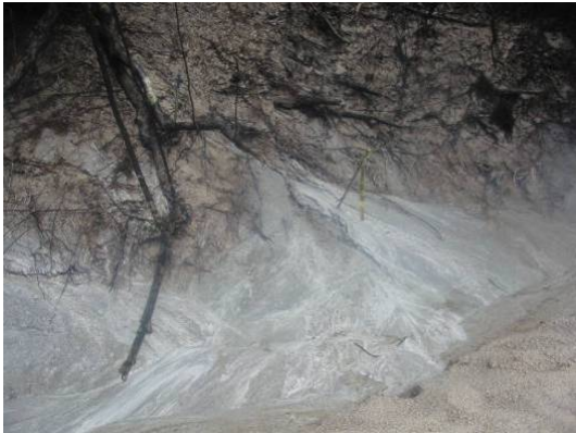
Photo 4-5 (left) New seepage flow at erosion pin site 3A. Seepage is likely associated with bank disturbance due to tree falls shown in following photo.
