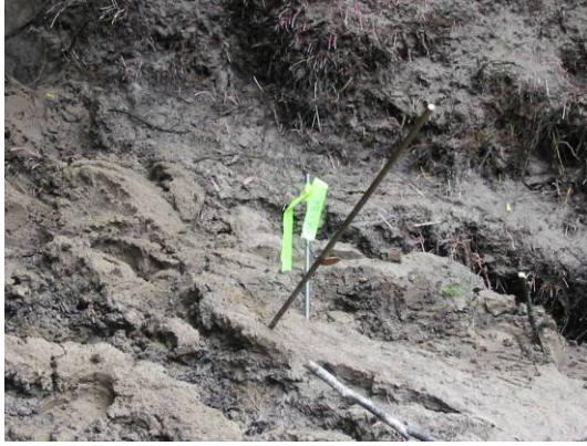
Photo 4-3 (left) Seepage erosion at erosion pin site 4B on March 17, 2007
