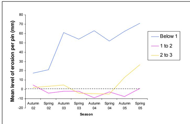
Figure 11.10. Mean erosion (+) and deposition (–) in zones 4 and 5 showing pins results grouped by turbine level.
