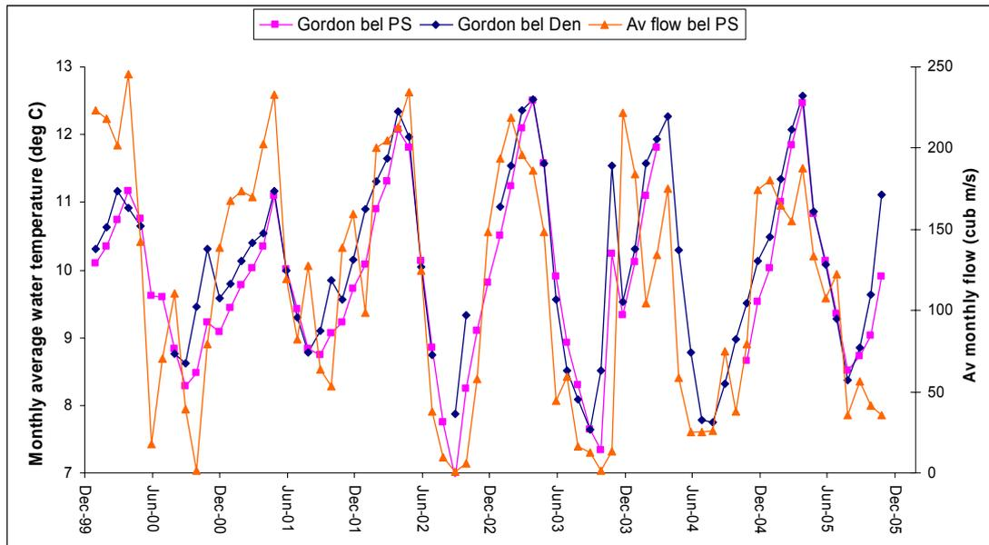
Figure 11.5. Average monthly flow rates superimposed on the water temperature curves.
