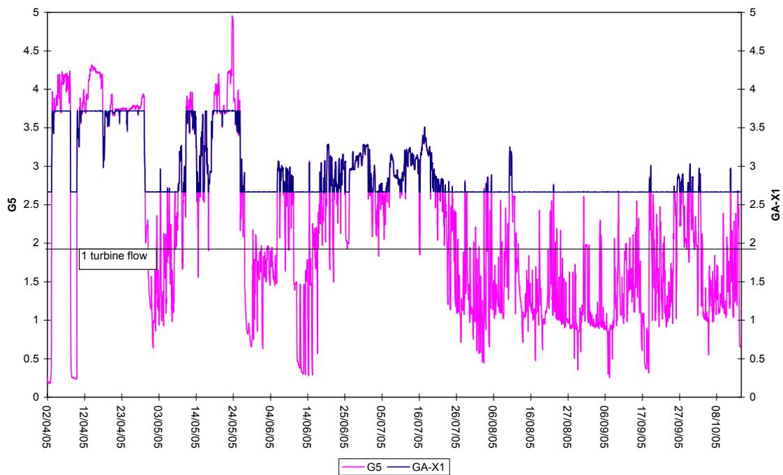
Figure 5.5. GA-X1 water level recorder with water levels from site 72 (G5) for comparison for the period of 2 April–15 October 2005. Data in metres above arbitrary zero datum.
