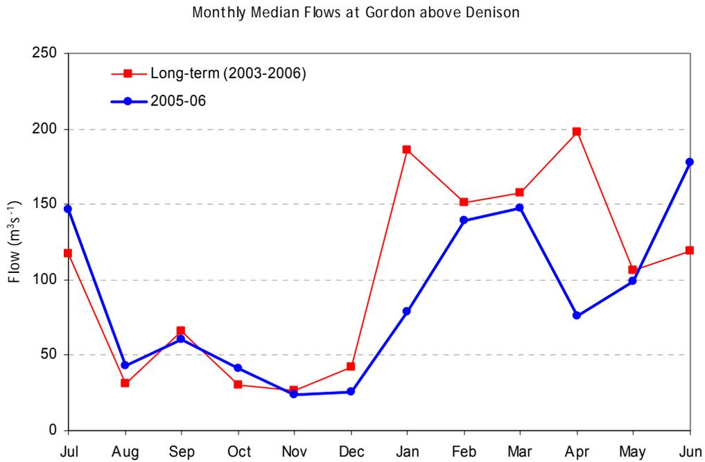
Figure 2.9. Median monthly flow at site 65 for 2005–06 compared with long-term median values.
