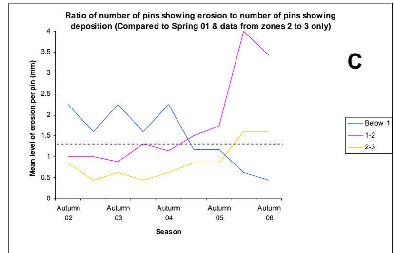
Figure 4.7. Erosion pin results grouped by turbine level for zones 2 and 3 only.
