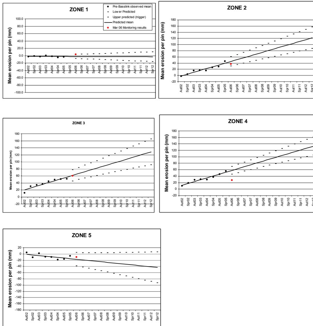
Figure 11.11. Graphical depiction of trigger values, showing linear trend fit to pre-Basslink monitoring results extended six years into the future, along with the 95<sup>th</sup> percentile confidence limits. The upper limit in each graph are the trigger values for that zone. Also shown are the March 2006 monitoring results. Note upper and lower limit of erosion scales differ, but each axis depicts 200 mm.
