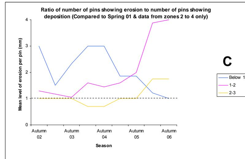
Figure 4.6. Erosion pin results grouped by turbine level.
