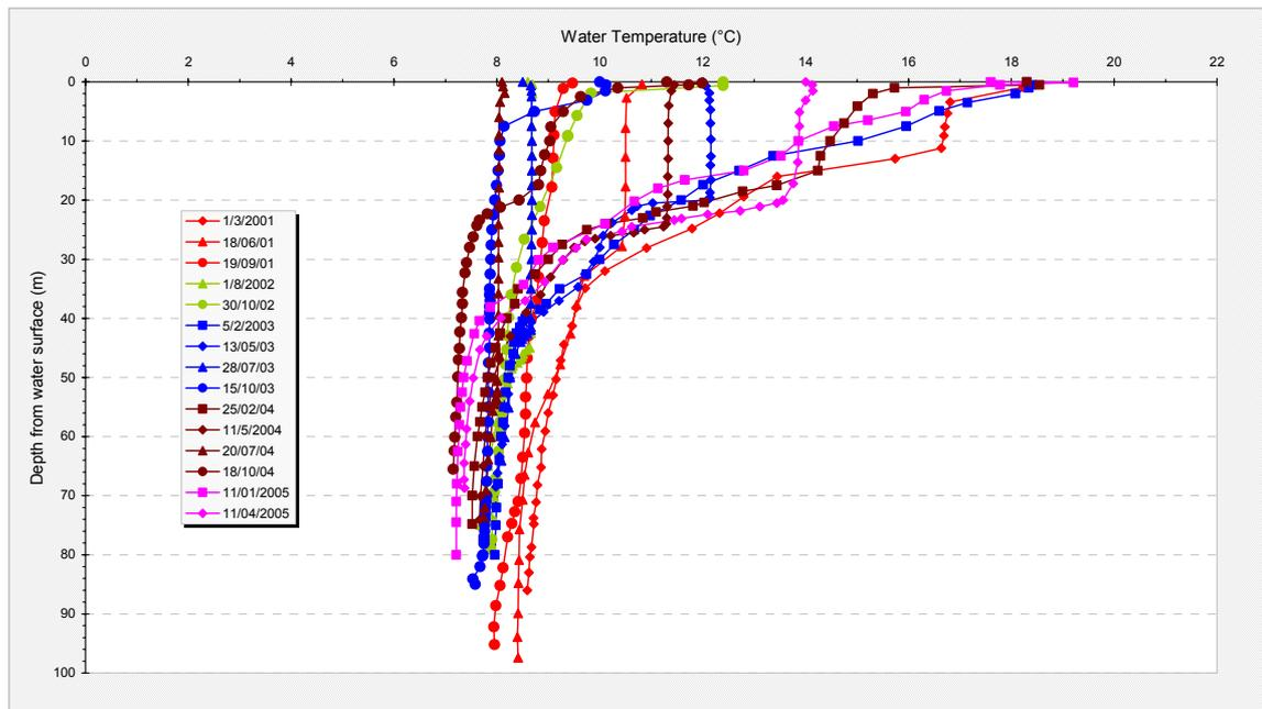
Figure 11.1. Temperature profiles from the Lake Gordon near the intake.
