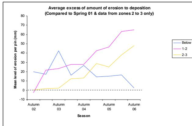
Figure 11.12. Erosion pin results grouped by turbine levels for zones 2 and 3 only showing autumn 2006 results along with pre-Basslink results.
