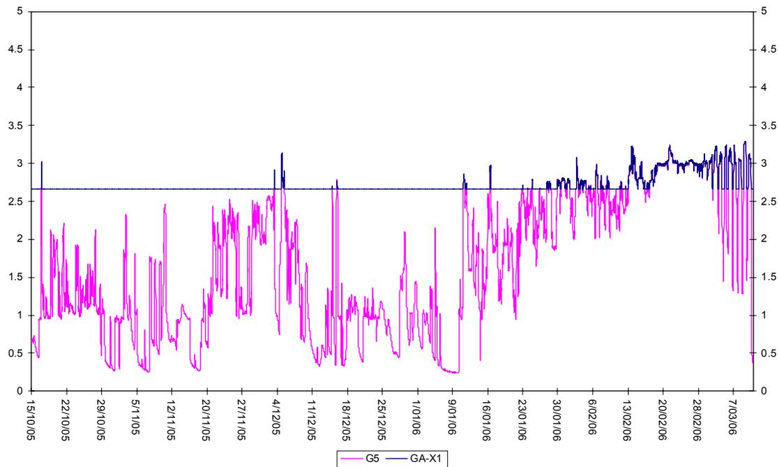
Figure 5.6. GA–X1 water level recorder with water levels from site 72 (G5) for comparison for the period 16 October 2005–11 March 2006. Data in metres above arbitrary local zero datum.
