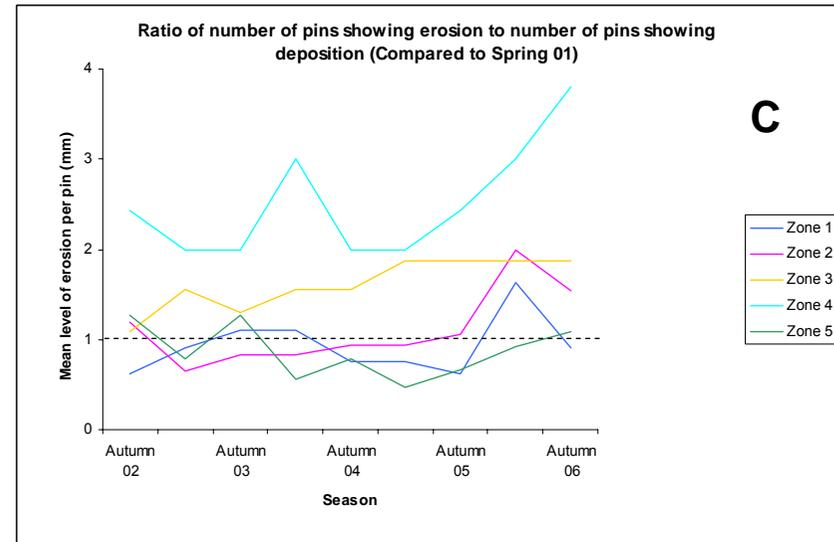
Figure 4.5. Erosion pin results grouped by zones. Monitoring occurs in autumn and spring of each year.
