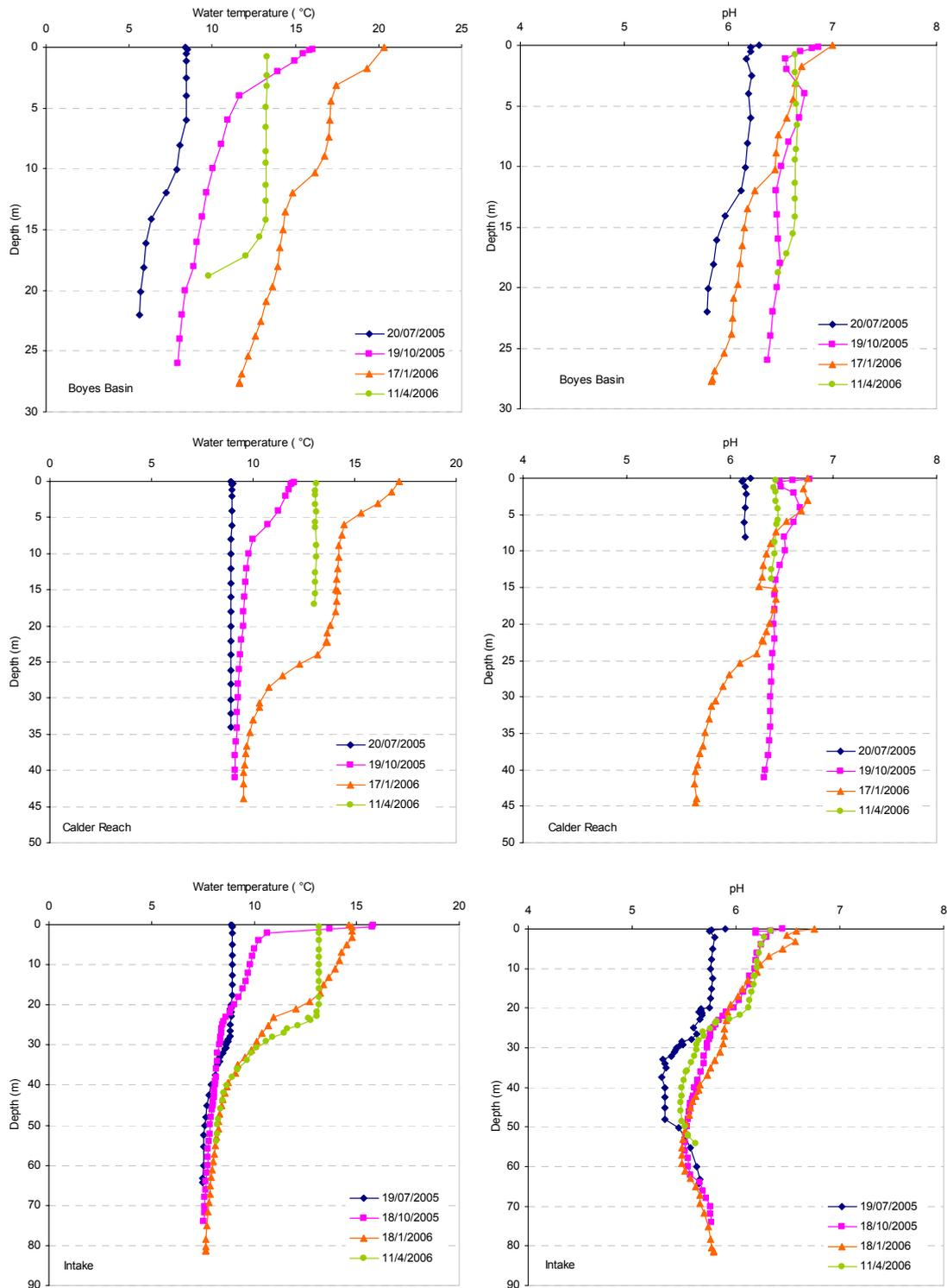
Figure 3.2. Depth profiles of water temperature (left) and pH (right) in Lake Gordon at Boyes Basin (top), Calder Reach (middle) and the power station intake (bottom) for 2005–06. Note that the intake gate level is at 254m ASL, and the intake depths were 22.1m (19 July 2005), 26.3m (18 October 2005), 29.6m (18 January 2006) and 27.2m (11 April 2006).
