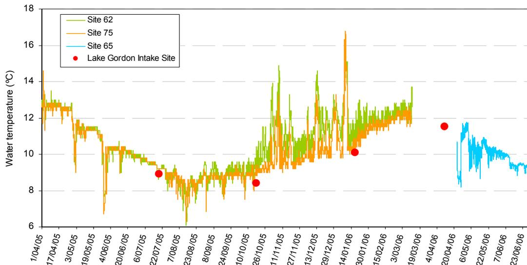
Figure 3.5. Water temperature data recorded for sites 75 (2km downstream of the tailrace), 65 (12km downstream of the tailrace) and 62 (15km downstream of the tailrace) from April 2005–June 2006. Note data from site 65 temperature data has been telemetered since its installation in April 2006, while sites 75 and 62 are downloaded manually from the datalogger and are only available until March.
