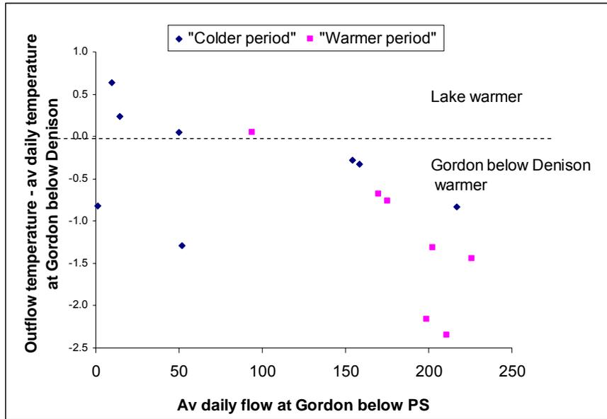
Figure 11.7. Difference between water temperatures at the Gordon below Denison River monitoring site and water temperature in Lake Gordon at the depth of the intake (254m) compared with flow rates from the power station.
