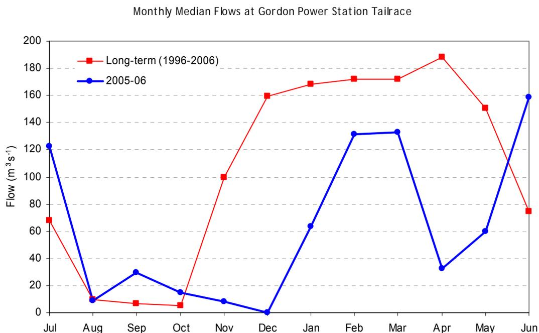
Figure 2.4. Median monthly discharge from the tailrace of the Gordon Power Station for 2005–06 compared with long-term median values.
