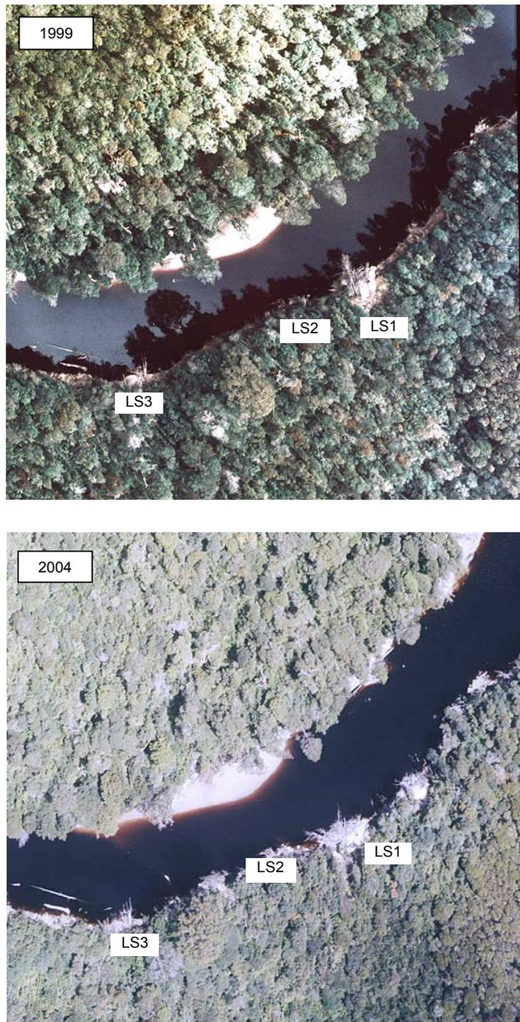
Photo 10.13. Aerial photo of zone 2 showing landslips in vertical cobble banks in 1999 (top) and 2004 (bottom).
