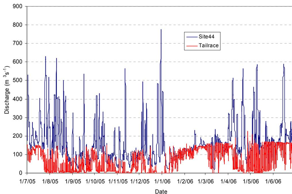
Figure 2.11. Flow recorded (hourly data) at site 44 (Gordon above Franklin) and the tailrace during 2005–06.
