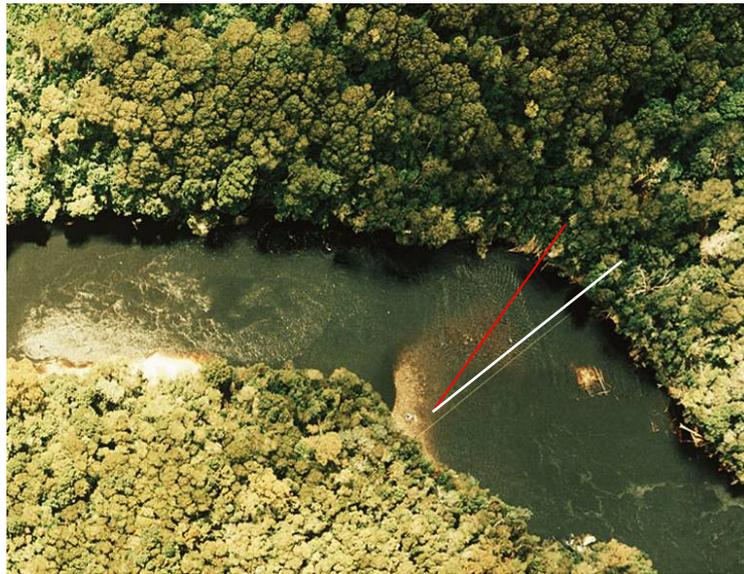
Photo 4.23. Aerial photo of site 11b showing difference in survey line in 2000 (white line) and in 2006 (red line) accounting for differences in channel profile.
