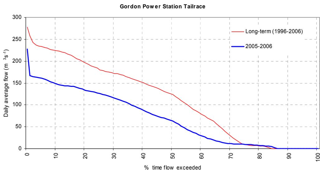
Figure 2.5. Duration curve for discharge from the power station tailrace for 2005–06.
