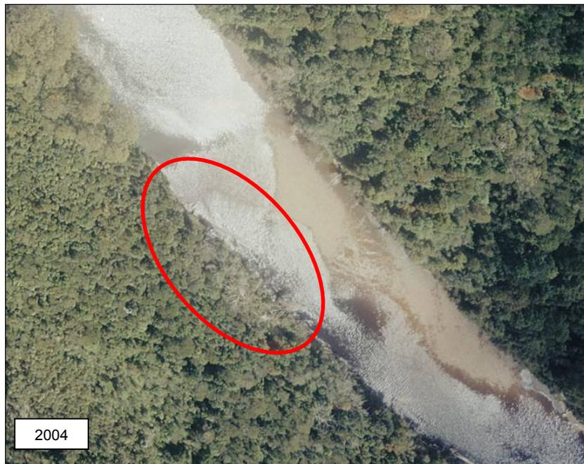
Photo 10.20. Zone 4 reach downstream of erosion pin site 4C, upstream from Bill Neilson Cave showing landslip on right bank. River flows from top to bottom of photo. Higher water level in 1999 is apparent from cobble bar exposure.
