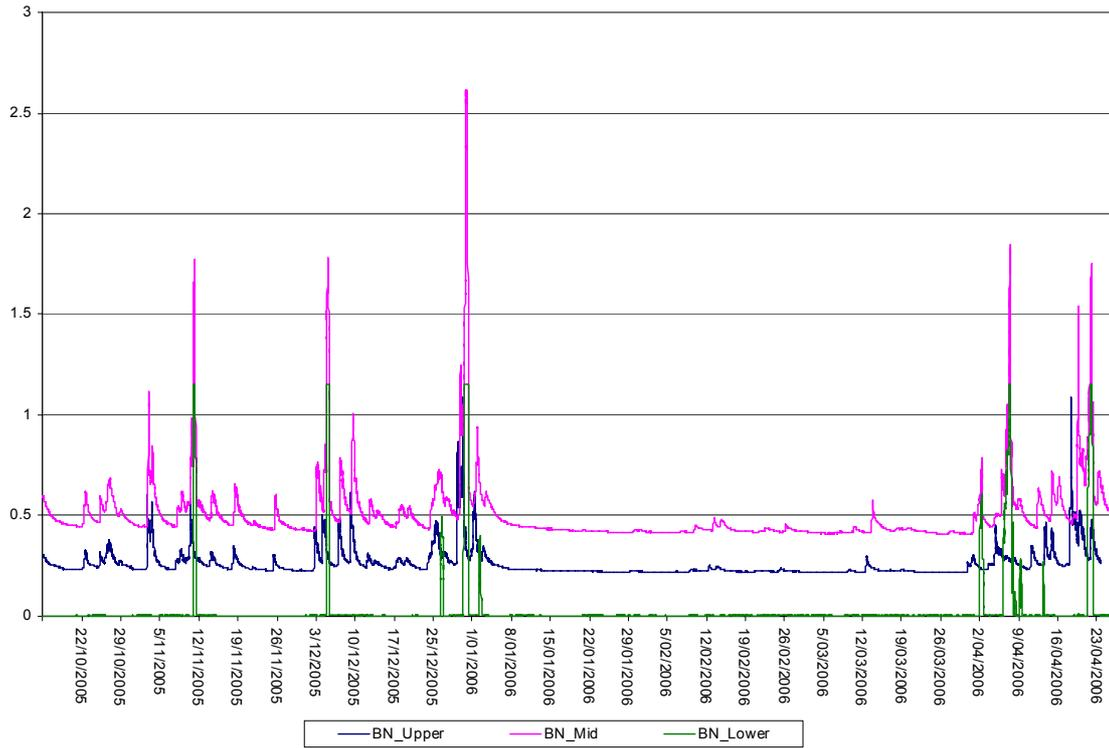
Figure 5.4. Bill Neilson Cave water level recorder data (BN\_Upper: cave stream only; BN\_Mid: cave stream and Gordon river water backflooding; BN\_Lower: Gordon River backflooding only) for the period 16 October 2005 to 11 March 2006.
