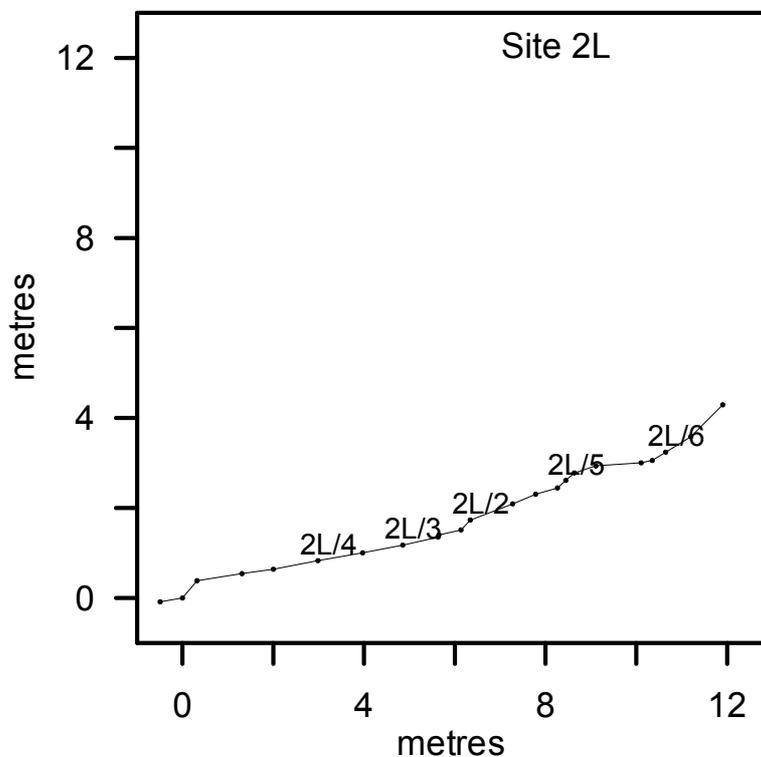
Figure 4.9. Profile of erosion pin site 2L, located on the right bank of the Gordon immediately upstream of the Splits (local datum).
