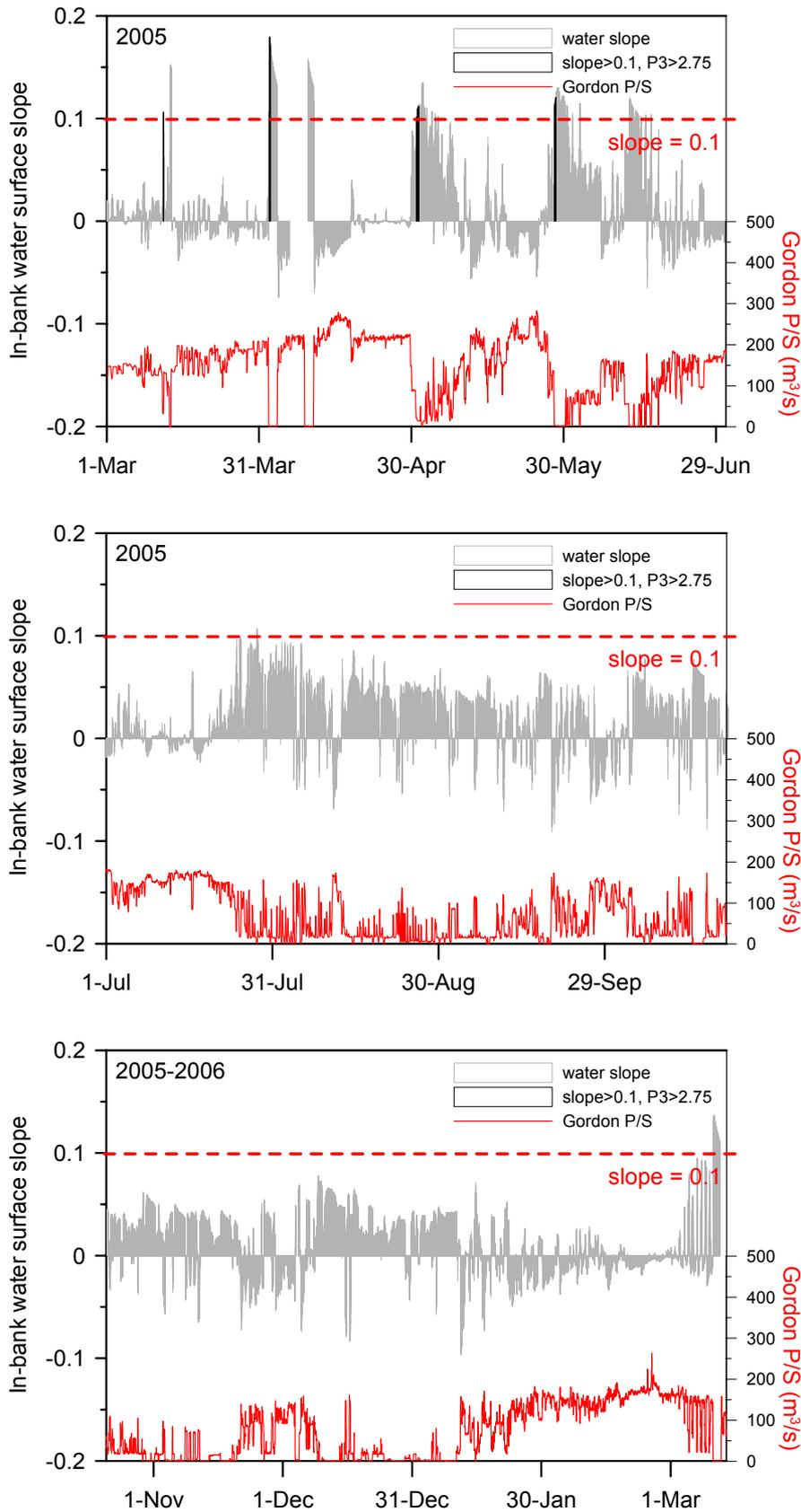
Figure 4.4. In-bank water surface slopes (upper) and discharge from Gordon Power Station (lower). Periods when water slopes exceed 0.1 and water level at probe 3 exceeds 2.75m are highlighted in black.
