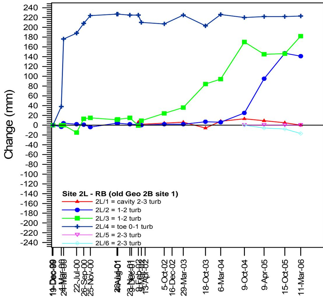
Figure 4.10. Erosion pin results from site 2K. Monitoring dates shown on x-axis.
