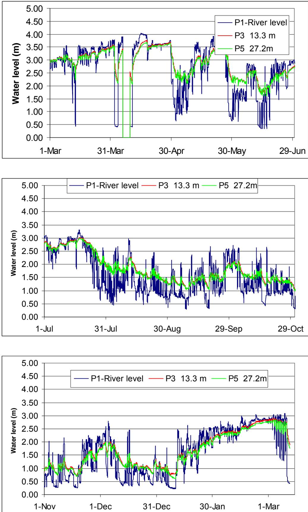
Figure 4.3. Piezometer data for probe 1 (river level) probe 3 (13.3m from bank) and probe 5 (27.2m from bank) between 1 March 2005 and 20 October 2005. Data interval is 15 min. Data missing between 6 and 9 April 2005.
