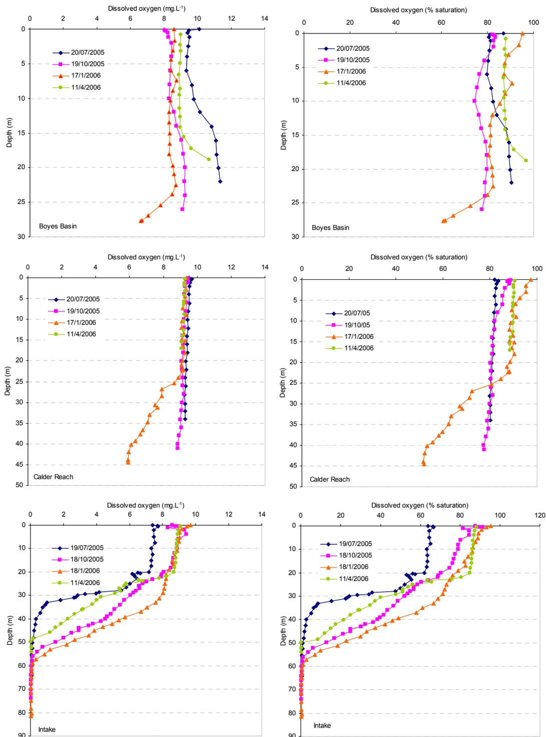
Figure 3.3. Depth profiles of dissolved oxygen concentration (left) and % saturation (right) in Lake Gordon at Boyes Basin (top), Calder Reach (middle) and the power station intake (bottom) for 2005–06. Note that the intake gate level is at 254m ASL, which corresponds to intake depths of 22.1m (19 July 2005), 26.3m (18 October 2005), 29.6m (18 January 2006) and 27.2m (11 April 2006).
