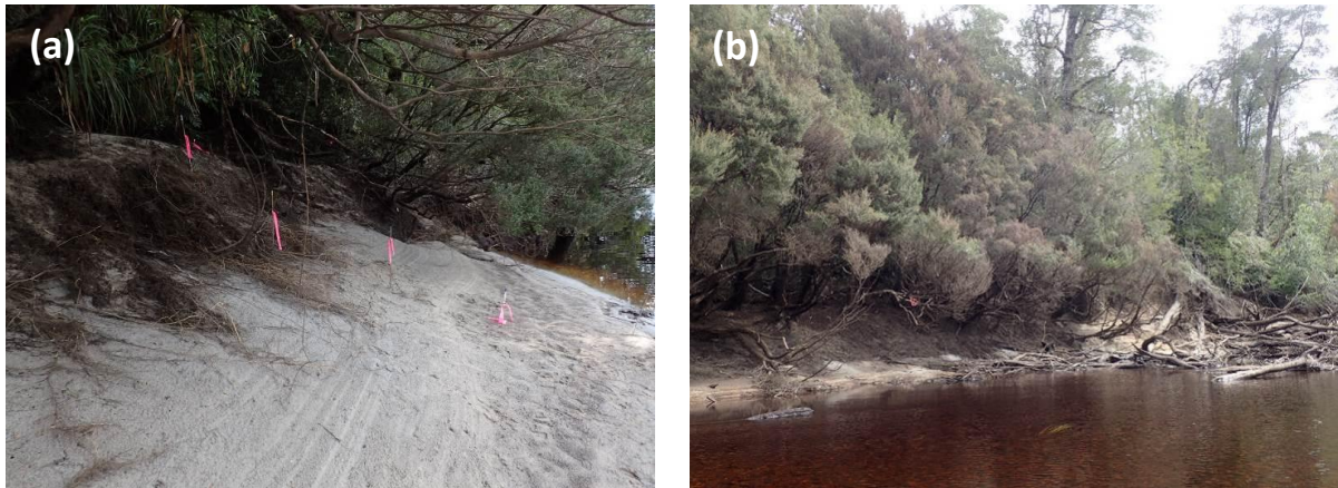
Figure 3-10: Scour and seepage features in zone 3. (a) Site 3E - scour on upper bank, seepage on lower bank; (b) site 3H - small sediment flows from under root mat.
