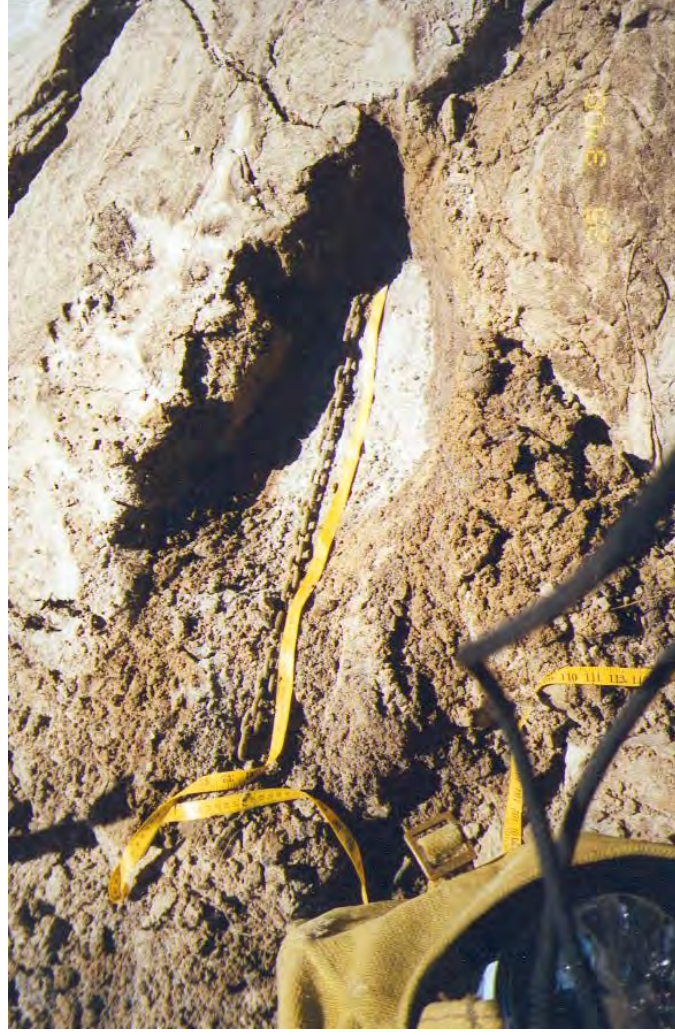
Photo 67. Scour chain in sediment flow in Zone 2
